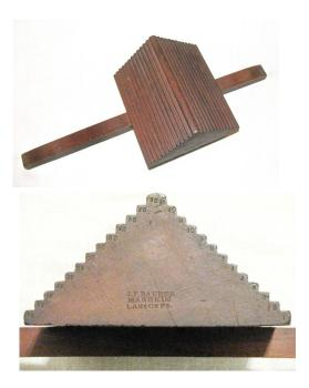
In early American homes, floor boards varied in widths and the floor board gauge was developed to make it possible for the carpenter to obtain the widest boards from stock, standardize the cuts and have boards of the same width fit end-to-end.
